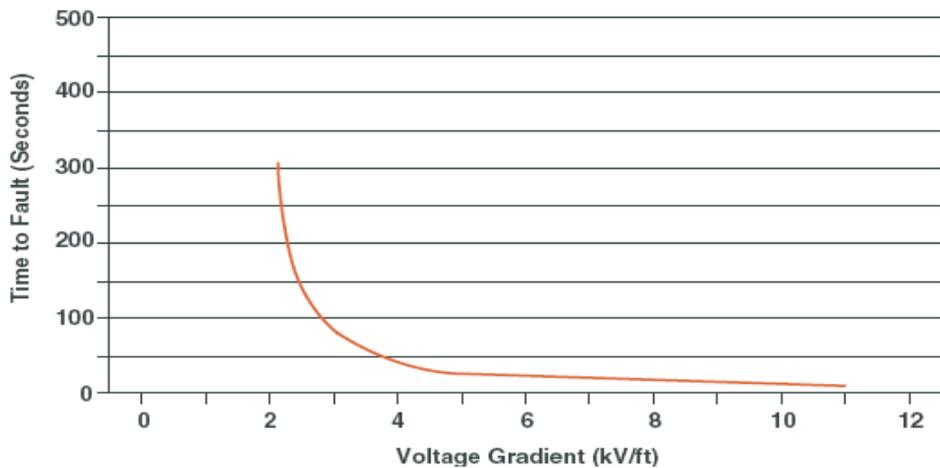
**Figure 5. Time-to-fault decreases as voltage stress gradient increases.**
