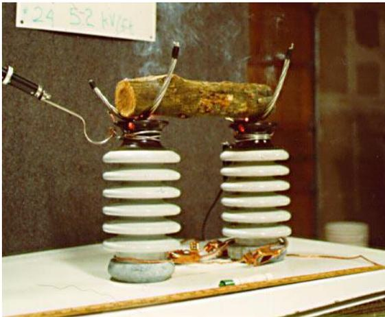
A high voltage test bench was assembled, with insulators positioned a fixed distance apart. Specimens were placed within saddles formed of aluminum wire, allowing consistent positioning for each test sequence. A variable output AC high potential transformer allowed for uniform testing at predetermined voltage levels.<sup>ii</sup>
