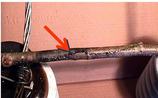
**Figure 4. A completed carbon path, fault occurred**
