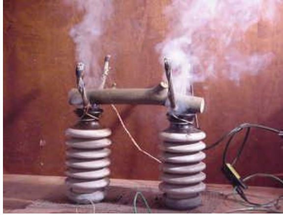
Figure 1: High voltage test setup showing two insulator specimens connected to a high voltage source, with smoke or steam rising from the specimens, indicating a fault or arcing event.
